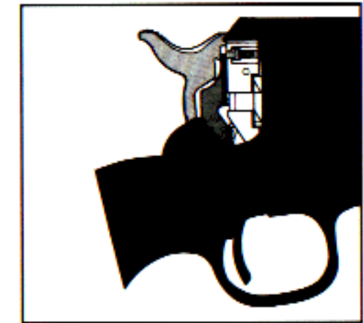
6. With trigger held fully rearward, the hammer actuates firing pin through transfer bar.
